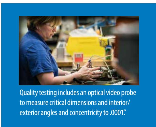
Quality testing includes an optical video probe to measure critical dimensions and interior/exterior angles and concentricity to .0001".
