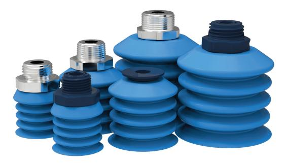
Cups of food contact materials (FCM) suitable for handling bread and pastries. In addition to threaded separable stainless steel and plastic fittings, all cups are available with a retainer clip which will fit standard bread depanners. The BBL cups can handle great differences in levels due to long bellows. Not suitable to use with deep vacuum levels.
