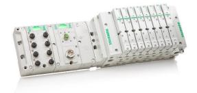
The 500 Series Valve Platform (501, 502 and 503) is fully integrated with the latest enhancements, including G3 and 580 Fieldbus. In addition, with the release of the 502 series it is possible to combine two valve sizes (503 & 502 or 502 & 501) in the same manifold assembly.
