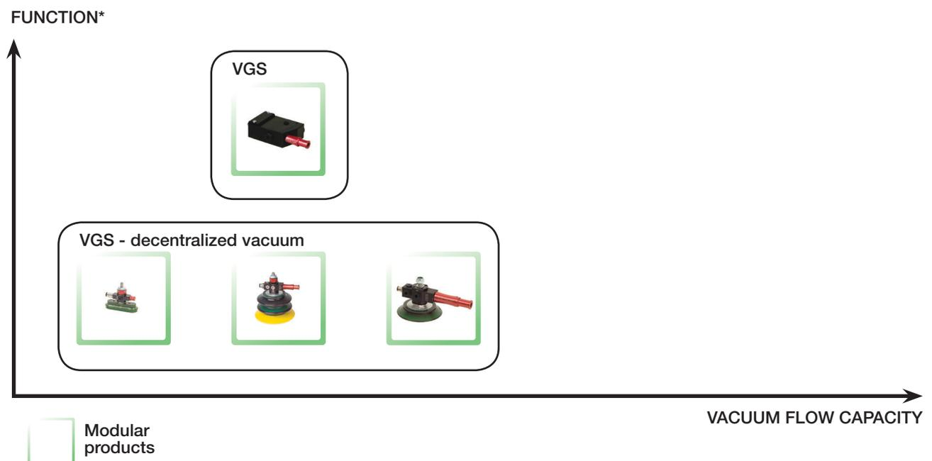
\* Function: Possibility to add functions, such as energy saving, release valve etc
