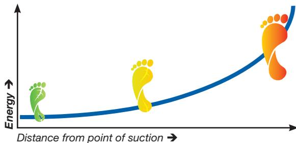
*The graph demonstrates the relationship between environmental impact and the distance of the pump from the point of suction.*
